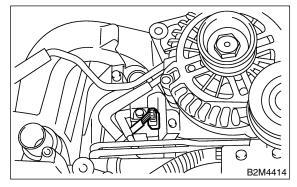
4) Remove bolt which installs purge control solenoid valve onto intake manifold.
