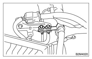
(4) Remove bolts which install power steering pump bracket.
