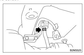
7) Remove fuel tank pressure sensor.
