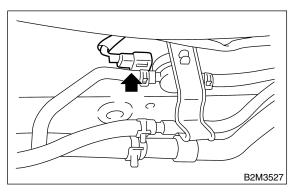
5) Disconnect two evaporation hoses from pressure control solenoid valve.
