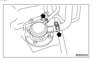
3) Remove nuts which install vent valve on fuel tank.
