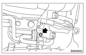
7) Disconnect evaporation hose (A) and remove drain valve (B).
