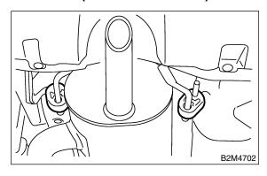
3) Remove front rubber cushion, and detach muffler assembly.
