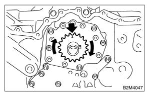
5) Install the idler sprocket. (Lower)
