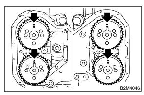
4) Rotate crankshaft sprocket clockwise to align "top mark" at 12 o'clock position as shown in the figure. (Piston # 1 is at TDC.)
