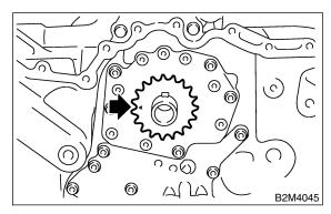
3) Using ST, align four key grooves on camshaft sprocket at 12 o'clock position as shown in the figure.
