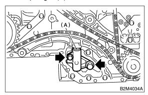
4) Remove chain guide. (Right-hand between cams)
