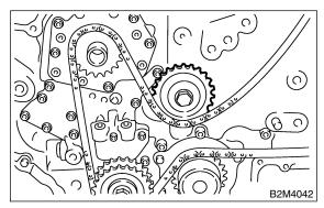
(4) Install chain guide. (Left-hand between cams)
