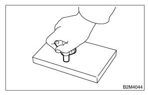
2) Using ST, align "top mark" on crankshaft sprocket at 9 o'clock position as shown in the figure.
