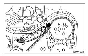
Remove chain guide. (Left-hand between cams)
