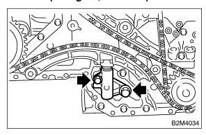
(7) Adjust the clearance between chain guide (RH) and chain guide (Center) to the range between 8.4 mm (0.331 in) to 8.6 mm (0.339 in). And install chain guide (Center).
