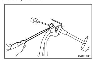
13) Disconnect accelerator cable stopper (A) from bracket.
