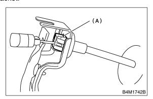
14) Separate accelerator cable and bracket.
