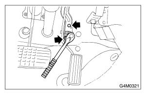
10) Disconnect grommet (A) from toe board.
