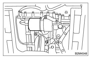
4) Get a new oil filter and apply a thin coat of engine oil to the rubber seal.
