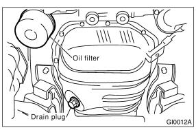
2) Get a new oil filter and apply a thin coat of engine oil to the seal rubber.
