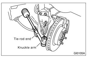
2) Check connections of knuckle ball joints for play, inspect for damage on dust seals, and check free play of ball studs. If castle nut is loose, retighten it to the specified torque, then tighten further up to 60° until cotter pin hole is aligned.
