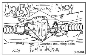
2) Check boot for damage, cracks or deterioration.
