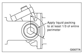
(4) Install lock nut. While holding adjusting screw with a wrench, tighten lock nut using ST.ST 926230000 SPANNER
