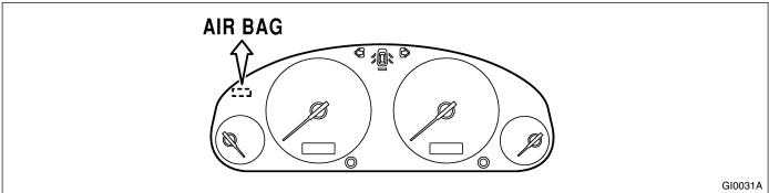
2) Turn the ignition switch ON, and connect the airbag diagnosis terminal of the service connector (located below lower cover) to the ground terminal.
