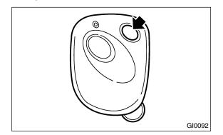
• Press the "UNLOCK/DISARM" button on the transmitter momentarily once again and check if all the doors including the rear gate on wagon are unlocked.
