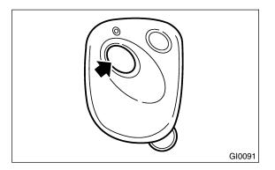
• Press the "UNLOCK/DISARM" button on the transmitter momentarily once and check if the driver's door is unlocked, the horn chirps twice and the dome light illuminates.
