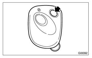
• Press the "UNLOCK/DISARM" button on the transmitter momentarily once again and check if all the doors including the rear gate on wagon are unlocked.
