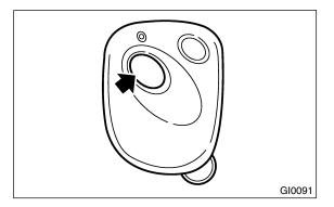
• Press the "UNLOCK/DISARM" button on the transmitter momentarily once and check if the driver's door is unlocked, the horn chirps twice, the parking lights flash twice, the dome light illuminates and the security indicator light goes off to ensure that the system has been brought into the disarming state.
