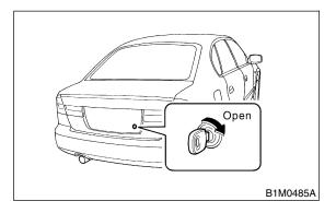
• Set the trunk lid release lever to the cancel position, and check that the trunk lid can only be opened with the key.
