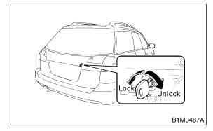
• Operate the power door locking witch to check that the rear gate is locked and unlocked normally.
