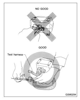
• Do not drop the airbag modulator parts, subject them to high temperature over 93°C (199°F), or let water, oil, or grease get on them; otherwise, the internal parts may be damaged and reliability greatly lowered.
