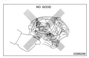
After removal, keep the airbag module with the pad facing upward on a dry, clean, and flat surface away from heat and light sources, and moisture and dust.
