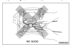
• The removed front seat with the airbag module must be kept at least 200 mm (8 in) away from walls and other objects.
