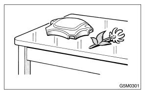
• Do not check continuity of the airbag module (driver, passenger, and side, pretensioner).
