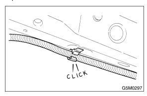
Do not allow water or oil to come in contact with the connector terminals. Do not touch the connector terminals.
