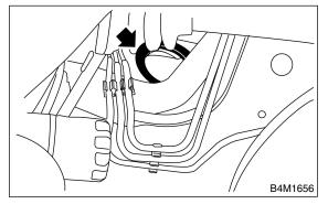
2) Insert end of steering shaft into toe board grommet.
