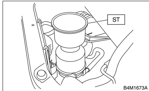
2) Jack-up vehicle and support it with safety stands, then turn steering wheel with engine stopped.
