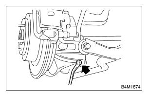
3) Remove bolts which secure stabilizer to sub frame.
