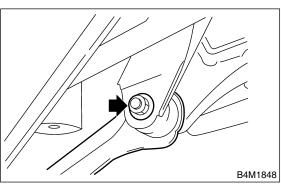
4) Remove bolts which secure link front to rear arm and detach link front.
