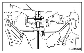
8) After removing bolts, remove sub frame and support sub frame from vehicle body.
