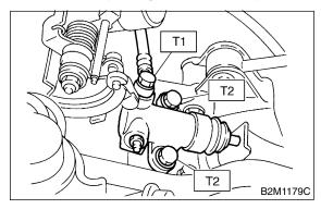
2) After bleeding air from operating cylinder, ensure that clutch operates properly. <Ref. to CL-20, Clutch Fluid Air Bleeding.>
