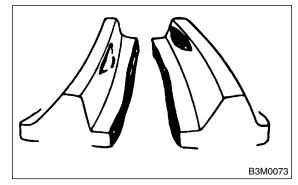
• The drive pinion shim selected before is too thin. Increase its thickness.
