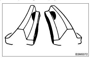
• The drive pinion shim selected before is too thick.
