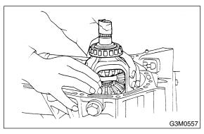
7) Remove differential side retainers using ST. ST 499787000 WRENCH ASSY
