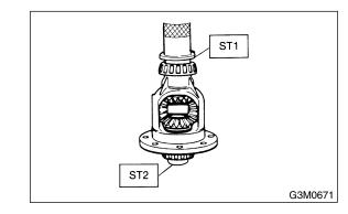
5) Install hypoid driven gear to differential case using twelve bolts.
