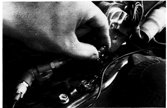
Removing FWD Fuse
