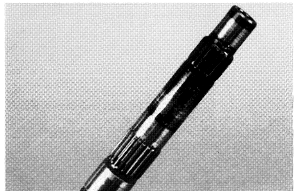
Discolored Input Shaft
