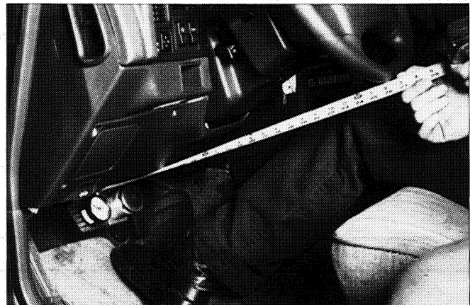
Measuring Brake Pedal Travel
