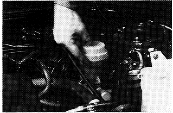
Checking Brake Fluid Level
