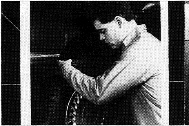
Checking for Brake Drag
