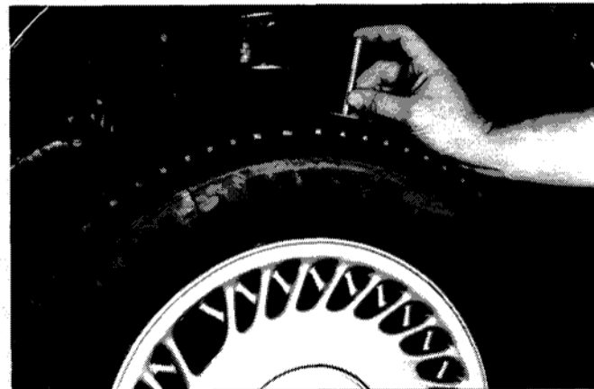
Checking Tread Depth
