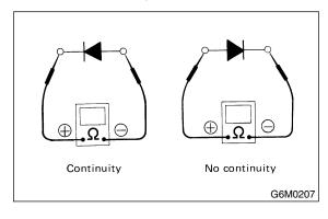
3) Symbol "OOO" indicates that continuity exists between two points or terminals. For example, when a switch position is "3", continuity exists among terminals 1, 3 and 6, as shown in table below.
