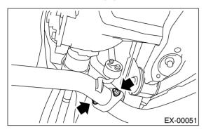
2) Remove the rubber cushions, and detach the muffler.
