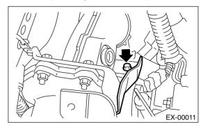
11) Place the turbocharger upper cover, and tighten the bolts which install the upper side of upper cover.
