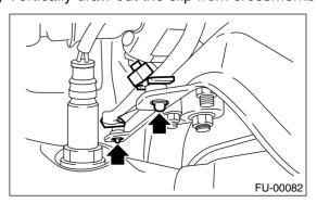
15) Separate the center exhaust pipe from rear exhaust pipe.
