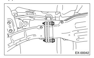
16) Remove the bolt which holds the center exhaust pipe bracket to transmission.
