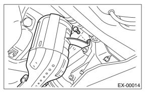
8) Tighten the bolt which holds the center exhaust pipe to hanger bracket.
