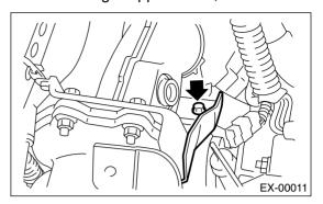
11) Separate the center exhaust pipe from turbocharger.
