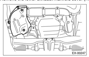
6) Remove the nuts which hold the front exhaust manifold to joint pipe.
