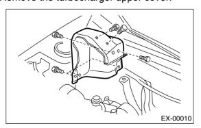
10) Remove the bolts which install the lower upper side of turbocharger upper cover, and remove it.
