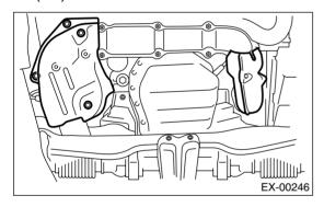
6) Remove the nuts and bolts which hold the front exhaust pipe assembly to turbocharger joint pipe.
