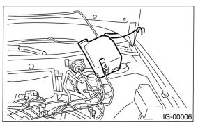
5) Disconnect the connector from ignition coil.
