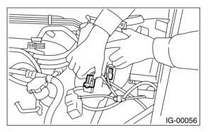
3) Remove the two bolts which hold the washer tank, then take the tank away from the working area.
