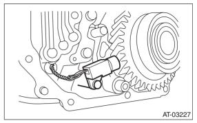
9) Remove the front vehicle speed sensor through the hole of AT transmission main case.
