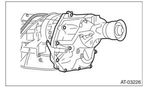
7) Install the rear vehicle speed sensor.
