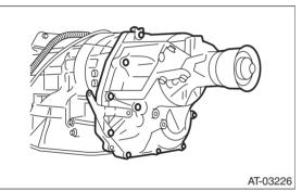
4) Remove the center differential carrier. <Ref. to 5AT-74, REMOVAL, Center Differential Carrier.>
