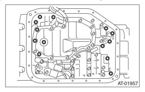
24) Remove the bolt securing harness of transmission main case.
