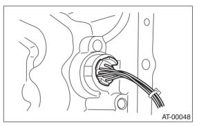
2) Install the securing bolt of transmission main case.
