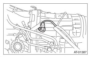
20) Remove the rear vehicle speed sensor.
