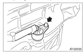
3) Install the control valve body.
