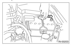
2) Remove the harness securing bracket.
