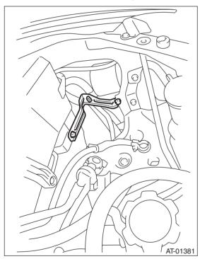
3) Using the ST, remove the ATF filter. ST 498545400 OIL FILTER WRENCH
