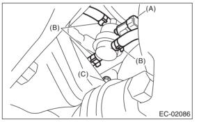
7) Remove the pressure control solenoid valve along with the bracket.
