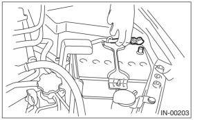
2) Disconnect the connector and evaporation hose of the purge control solenoid valve, then remove the purge control solenoid valve.
