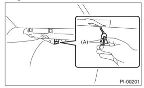
6) Connect the Subaru Select Monitor to data link connector located in the lower portion of the instrument panel (on the driver's side).
