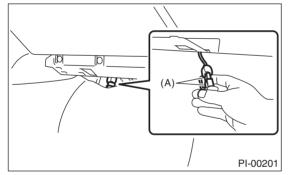
4) Connect the general scan tool to data link connector located in the lower portion of the instrument panel (on the driver's side).
