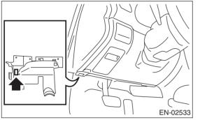
3) Using the general scan tool, call up DTC and freeze frame data.
