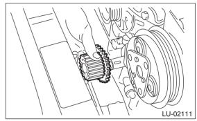
14) Remove the bolts which install oil pump onto cylinder block.
