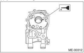
4) Install the oil pump to cylinder block. Be careful not to damage the oil seal during installation.
