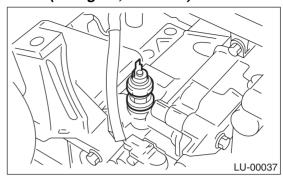
3) Connect the terminal to the oil pressure switch.
