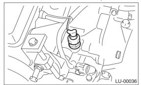
3) Remove the oil pressure switch.
