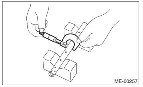
2) If the oil clearance exceeds the limit, replace the valve rocker arm or shaft, whichever shows the greater amount of wear.
