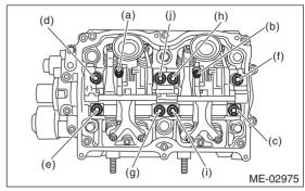
(3) Remove the valve rocker assembly.
