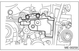
9) Remove the camshaft position sensor support. (LH side only)
