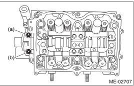
(2) Equally loosen the bolts (c) through (j) all the way in alphabetical sequence.
