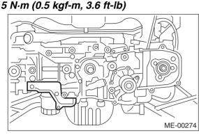
12) Install the cam sprocket. <Ref. to ME(H4SO)-
