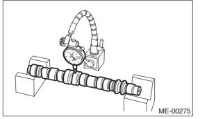
2) Check the journal for damage and wear. Replace if faulty.
