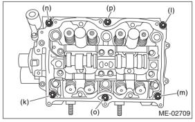
(4) Remove the camshaft cap.
