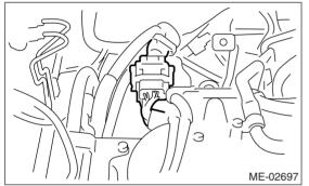
4) Disconnect the connector from the oil switching solenoid valve.
