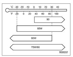
SAE viscosity No. and applicable temperature
