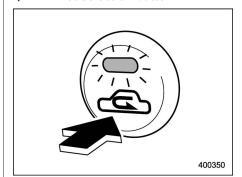
ON position (Recirculation): Interior air is recirculated inside the vehicle.
