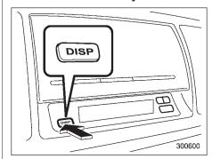
With the ignition switch in the "ON" position, each successive push of the "DISP" button toggles the display in the following sequence:
