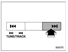
Briefly press the """ side of the TUNE/ TRACK button to skip to the beginning of the next track/file (track). Each time the button is pressed, the indicated track/file (track) number will increase.
