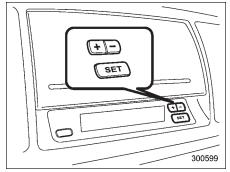
To adjust the time shown by the clock, press the "+" button or the "-" button. The indicated time will change in one-minute increments. If you keep the button pressed, the rate at which the indicated time changes will speed up.
