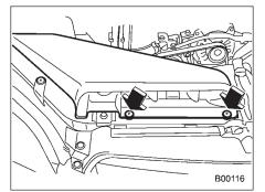
1. Use a screwdriver to undo the clips on the air intake duct, then remove the air intake duct.
