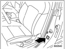
The load capacity of your vehicle is determined by weight, not by available cargo space. The maximum load you can carry in your vehicle is shown on the vehicle placard attached to the driver's
