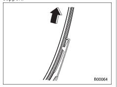
2. Pull the blade rubber assembly out of the plastic support.
