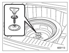
6. Turn the attaching bolt counterclockwise, then take spare tire out.
