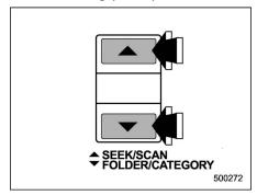
If you press the "\( \bigcup \)" or "\( \bigcup \)" side of the SEEK/SCAN button for 0.5 second or longer, the radio will switch to scan mode. In this mode, the radio scans through the radio band until a station is found. The radio will stop at the station for five seconds while displaying the frequency, after which scanning will continue until the entire band has been scanned.
