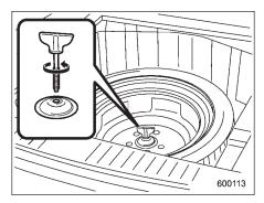
6. Turn the attaching bolt counterclockwise, then take the spare tire out.
