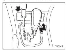
If you inadvertently have turned the ignition switch to the "OFF" position with the selector lever in the "N" position, proceed as follows. By referring to the "Shift lock release" section in this chapter, remove the shift lock release cover. Then, with the screwdriver inserted into the hole, move the selector lever to the "P" position. If the selector lever reverse inhibiting function fails, have the vehicle inspected by the nearest SUBARU dealer.
