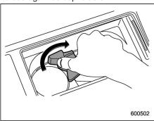
Insert the protrusion on the back of the divider plate into the hole in the center of the console box. Grasp the divider plate at the base, and turn it clockwise to fit it.
