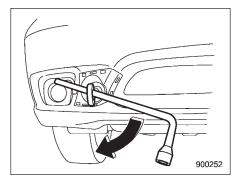
6. Tighten the towing hook securely using a wheel nut wrench.
