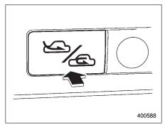
Select air flow by pushing the air inlet selection button " "."
