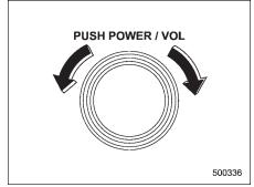
The volume control dial normally functions as a volume control. This dial becomes a control for Bass, Midrange, Treble, Fader or Balance when you select the appropriate tone and balance control mode.
