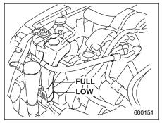
Check the coolant level at each fuel stop.
