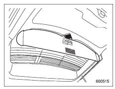
Rotate the rear gate board toward you until its top touches the rear gate panel.
