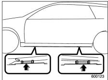
8. Place the jack under the side sill at the front or rear jack-up point closest to the flat tire.
