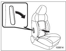
Pull the lever forward or backward. Pulling the lever forward will increase the amount of support for your lower back.
