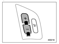
Press the "+" button to increase the volume. Press the "-" button to reduce the volume.
