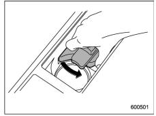
Grasp the dual cupholders' divider plate at the base. Turn it counterclockwise to remove it.
