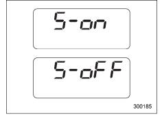
It is possible to activate or deactivate the movement of the meter needles and gauge needles that takes place when the ignition switch is turned to the "ON" position.
