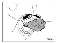
The key can be turned from "ACC" to "LOCK" only when the selector lever is in the "P" position.
