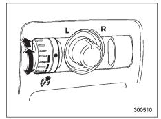
The brightness of clock display, audio, air conditioner, information display and instrument panel illumination dims when the light switch is in the "≥oof" or "≣()" positions. You can adjust brightness of the instrument panel illumination for better visibility.
