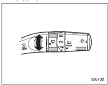
When the wiper switch is in the """ position, turn the dial to adjust the operating interval of the wiper.
