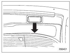
To close the rear gate, lower it slowly and push down firmly until the latch engages. The rear gate can be lowered easily if you pull it down holding the recessed grip.
