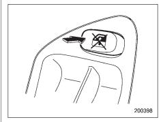
To lock the passengers' windows, push the lock switch. When the lock switch is in the "LOCK" position, the passengers' windows cannot be opened or closed. Press the switch again to cancel the passengers' window locking.
