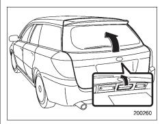
The rear gate can be locked and unlocked using either the keyless entry system or the power door locking switch.
