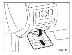
Open the lid that is located above the hood release knob and pull it toward you to remove it.
