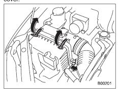
4. Unsnap the two clamps holding the air cleaner case cover.
