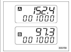
This meter displays the two trip meters when the ignition switch is in the "LOCK", "ACC" or "ON" position.
