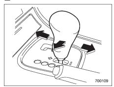
With the vehicle either moving or stationary, move the selector lever from the "D" position to the manual gate then move it to the "+" end or "-" end of the manual gate to select manual mode.
