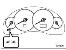
SRS airbag system warning light (Nonturbo models)
