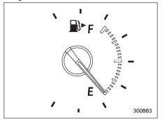
The rim of the fuel gauge flashes five times when the amount of remaining fuel reaches 2.6 US gal (10 liters, 2.2 lmp gal). If you turn the ignition switch to the "LOCK" position and back to the "ON" position, the rim will again flash five times.
