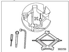
Screwdriver Towing hook Wheel nut wrench
