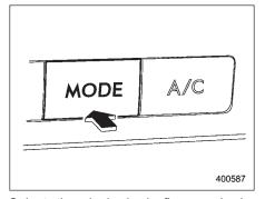
Select the desired air flow mode by pushing the air flow mode selection button. The selected air flow mode is shown by the display.
