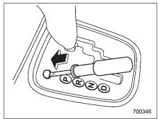
3. Remove the cover by prying on the edge with a flat-head screwdriver.
