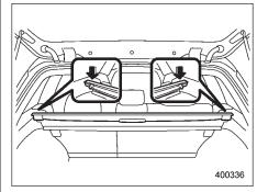
To install the cover housing, insert both ends of the cover housing into the retainers.
