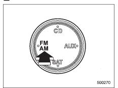
Push the "FM AM" button when the radio is off to turn on the radio.
