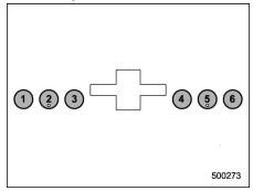
1. Use the disc select button to select the disc to be ejected.
