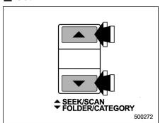
The scan mode lets you listen to the first 10 seconds of each track/file (track) in succession. Press the "\( \Lambda \)" side of the SEEK/SCAN button for 0.5 second or longer to start scanning upward beginning with the track/file (track) following the currently selected one. Press the "\( \P \)" side of the button to start scanning downward beginning with the track/file (track) preceding the currently selected one.
