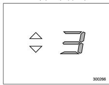
When the manual mode is selected, the gear position indicator (which shows the current gear selection) and the upshift/ downshift indicator light up. (Refer to the "Automatic transmission - 4-speed" or "Automatic transmission - 5-speed" section in chapter 7.)
