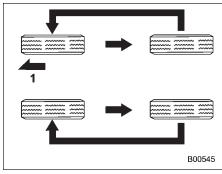
Vehicles equipped with unidirectional tires 1) Front
