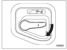
To open the trunk lid from inside the trunk. press the yellow handle downward as indicated by the arrow on the handle. This operation unlocks the trunk lid. Then, push up the lid.
