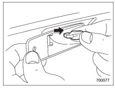
3. Pull the bulb out of the socket. Install a
