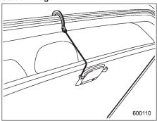
1. Open the lid and hang the hook provided on the under side of the lid on
