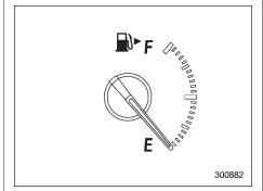
The fuel gauge shows the approximate amount of fuel remaining in the tank. When the ignition switch is in the "LOCK" or "ACC" position, the fuel gauge shows "E" even if the fuel tank contains fuel.
