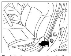
Check the tire pressures when the tires are cold. Use a pressure gauge to adjust the tire pressures to the values shown on the tire placard. The tire placard is located on the door pillar on the driver's side.
