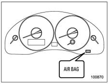
SRS airbag system warning light (Turbo models)
