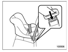
8. To remove the child restraint system, press the release button on the seatbelt buckle and allow the belt to retract completely. The belt will return to the ELR mode.
