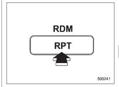
To repeat the currently playing disc/folder, press the "RPT" button twice while a track/ file (track) is playing. The display will show "D-RPT" for non-MP3/WMA disc, "F-RPT" for MP3/WMA folder. And the disc/folder will be played repeatedly.
