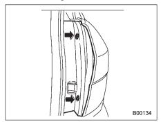
1. Using a Phillips screwdriver, remove the upper and lower screws.
