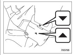
4. After fastening the seatbelt, make sure that the "\overline" mark on the connector (tongue) and the "A" mark on the buckle face outwards.
