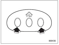
2. Press and hold the two outside buttons until the HomeLink® indicator light begins to flash (after 20 seconds). Release both buttons.
