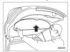
Insert (tipped at an angle) the hooks on the rear gate board into the holes in the rear gate panel.
