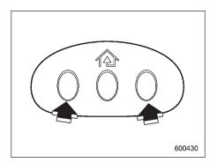
2. Press and hold the two outside HomeLink® buttons until the indicator light begins to flash (after 20 seconds). Release both buttons.
