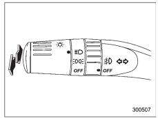
To change from low beam to high beam, push the turn signal lever forward. When the headlights are on high beam, the high ment panel is also on.
