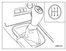
The shift pattern is shown on the shift lever knob. When shifting from 5th gear to reverse gear, first return the shift lever to the neutral position then shift into reverse gear.
