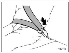
Push the release button of the center seatbelt buckle (on the left-hand side) to unfasten the seatbelt.
