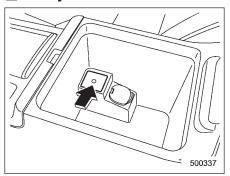
By connecting a commercial audio product to the vehicle, such as portable audio player, you can hear its sound via the vehicle's speaker.
