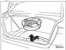
**Sedan:** To take out the jack and maintenance tools, open the floor cover and remove the bucket from the center of the spare tire. Then, take the jack out of the bucket.
