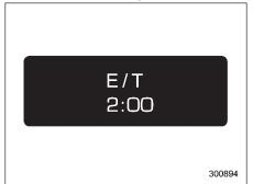
After 2 hours have passed for the journey time, the display indication flashes "E/T 2:00" at the center of the display for 3 seconds and gives a notice to the driver to take a rest. After 3 seconds, it returns to its original indication of the outside temperature and journey time.
