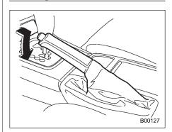
Check the parking brake stroke according to the maintenance schedule in the "Warranty and Maintenance Booklet". When the parking brake is properly adjusted, braking power is fully applied by pulling the lever up five to six notches gently but firmly (approximately 44 lbs, 196 N, 20 kg). If the parking brake lever stroke is not within the specified range, have the brake system checked and adjusted at your SUBARU dealer.
