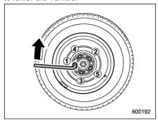
14. Use the wheel nut wrench to securely tighten the wheel nuts to the specified torque, following the tightening order in the illustration.
