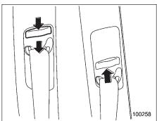
The shoulder belt anchor height should be adjusted to the position best suited for the driver/front passenger. To lower the anchor height, push the release button and slide the anchor down. To raise the anchor height, slide the anchor up. Pull down on the anchor to make sure that it is locked in place.
