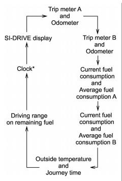
\*: Only for vehicles equipped with a navigation system
