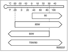
SAE viscosity No. and applicable temperature
