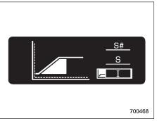
The Intelligent (I) mode provides wellbalanced performance with greater fuel efficiency and smooth driveability without stress. Power delivery is moderate during acceleration for maximum fuel efficiency.
