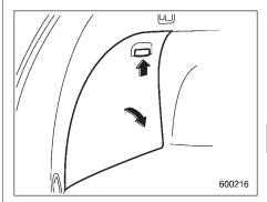
A stowage box is located on each side of the cargo area. You can access each one by pushing up and pulling the knob on the
