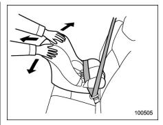
6. Push and pull the child restraint system forward and from side to side to check if it is firmly secured.
