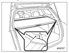
To extend the cover, pull the end of the cover out of the housing, then insert its hooks into the catches as shown. To rewind it, unhook it from the catches and it will rewind automatically. You should hold on to the cover and guide it back into the cover housing while it is rewinding.
