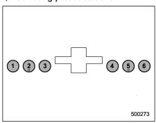
Presetting a station with a preset button allows you to select that station in a single operation. Up to six AM, FM1 and FM2 stations each may be preset.
