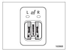
The seat heater is equipped in the front
