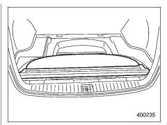
4. Stow the cover housing and rear gate board in the cargo area end.
