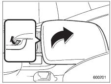
Pull up the lock release knob at the bottom of the front edge of the lid.
