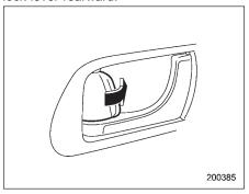
To unlock the door from the inside, rotate the lock lever forward.
