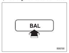
Each brief press of the "BAL" button changes control modes in the following sequence starting from volume control mode. (When the radio is first turned on, the control mode is in the volume control.)
