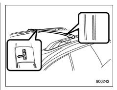
3. The crossbar with the 100 LBS Load Label attached onto it is the front crossbar. An arrow is marked on the back of the front crossbar for correct installation. Install the front crossbar so that the arrow faces the front of the vehicle.
