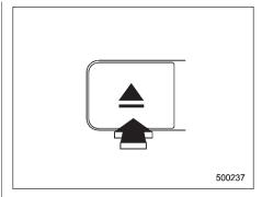
2. Briefly press the "\_\_\_" button. The selected disc will be ejected. The disc number indicator will flash at this time. When you remove the ejected disc, the disc number indicator will go off.
