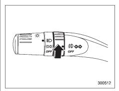
The front fog lights operate only when the light switch is in the "\( \bigcirc\)" position.
