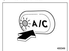
The air conditioner operates only when the engine is running.
