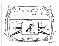
The cargo area is equipped with four tiedown hooks so that cargo can be secured with a luggage net or ropes.
