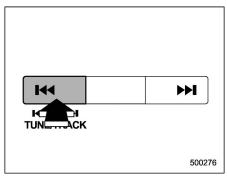
Briefly press the " side of the TUNE/ TRACK button to skip to the beginning of the current track/file (track). Each time the button is pressed, the indicated track/file (track) number will decrease.
