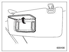
To use the vanity mirror, swing down the sun visor and open the vanity mirror cover. The light beside the vanity mirror comes on when the ignition switch is either in the "ACC" or "ON" position and the mirror cover is opened.
