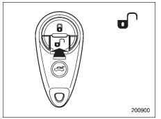
Press the " $\ \ \ \$ " button to unlock the driver's door. An electronic chirp will sound twice and the turn signal lights will flash twice. To unlock all doors and the rear gate (Station wagon), briefly press the "T" button a second time within 5 seconds.
