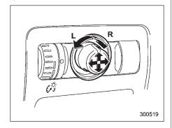
The remote control mirrors operate only when the ignition switch is in the "ON" or "ACC" position.
