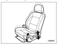
The height of the seat can be adjusted by moving the seat cushion adjustment lever up and down.
