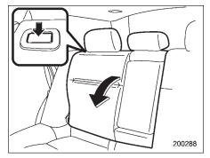
Unlock the seatback by pushing the release button and then fold the seatback down.
