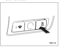
Pressing the switch to deactivate the Vehicle Dynamics Control system can facilitate the following operations:
