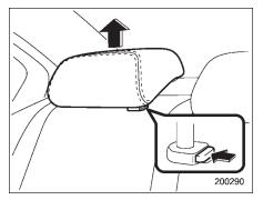
1. Remove the head restraint at the seating position where the child seat has been installed with the seatbelt or lower anchorages; lift up the head restraint while pressing the release button.
