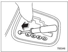
3. Remove the cover by prying on the edge with a flat-head screwdriver.
