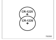
2. Remove the circuit board from the bottom half of the case and slide the white plastic battery holder out from under the battery tab releasing the batteries. Remove the old batteries and replace with new ones. Be sure to observe the (+) sign
