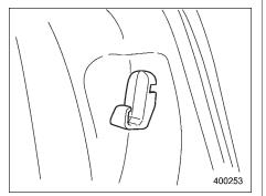
A shopping bag hook is attached to each inner side wall of the trunk near the trunk lid opening.
