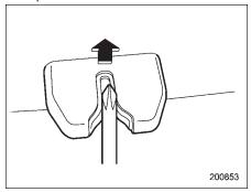
2. Use a screwdriver with a thin blade. Slide the screwdriver blade from the slit aperture of the lock assembly fully to the end until you hear a click.
