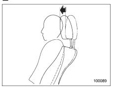
The front seats of your vehicle are equipped with active head restraints. They automatically tilt forward slightly in the
