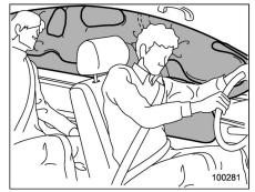
The SRS side airbag and SRS curtain airbag can function only when the ignition switch is in the "ON" position.
