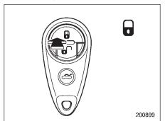
Press the "a" button to lock all doors and rear gate (Station wagon). An electronic chirp will sound once and the turn signal lights will flash once.
