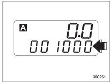
This meter displays the odometer when the ignition switch is in the "LOCK", "ACC" or "ON" position.
