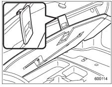
1. Lift the handle of the floor cover and hook the handle onto the trunk edge.
