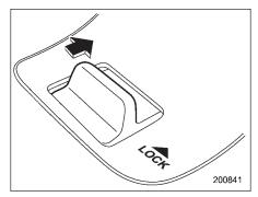
5. Before the electronic tone stops sounding, press the power door lock knob to the "LOCK" side the same number of times as the leftmost digit of the transmitter code. For example, press the lock knob eight times if the leftmost digit of the code is 8.
