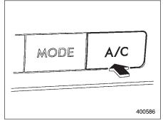
If the windshield starts to fog when the climate control system is operated in the AUTO mode, push the air conditioner button "A/C" to defog and dehumidify.
