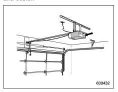
1. Locate the training button on the garage door opener motor head unit. The exact location and color of the button may vary by brand of garage door opener. If it is difficult to locate the training button, refer to your garage door opener's instruction manual.
