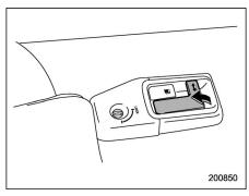
Pull the trunk lid release lever upward.
