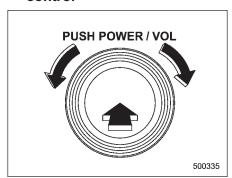
The dial is used for both power (ON/OFF) and volume control. The radio is turned ON and OFF by pushing the dial and the volume is controlled by turning the dial. The dial can also be used for tone and balance adjustment.
