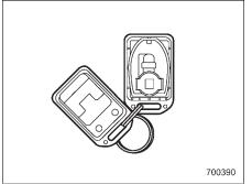
1. Carefully pry the remote control halves apart using a small flathead screwdriver.
