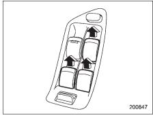
To close the window, pull the switch up and hold it until it reaches the desired position.
