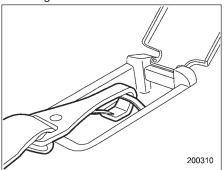
3. Fasten the top tether hook of the child restraint system to the appropriate upper anchorage.
