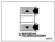
If you press the "▲" or "▼" side of the SEEK/SCAN button briefly, the radio will automatically search for a receivable station and stop at the first one it finds. This function may not be available, however, when radio signals are weak. In such a situation, perform manual tuning to
