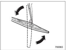
2. Turn the wiper blade assembly counterclockwise.
