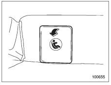
Remove the two covers from the selected side of the rear seatback to expose the anchorages (bars) to be used for installation of the child restraint system.
