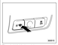
The windshield wiper deicer operates only when the ignition switch is in the "ON" position.
