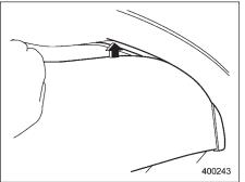
Fit the top of the rear gate board into the groove in the rear gate panel.
