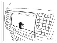
To open the center panel compartment, pull up the edge of the bottom of the panel
