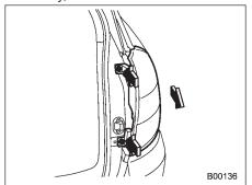
3. Remove the upper and lower screws. Then, slide the rear combination lamp assembly to the rear and remove it from the vehicle.
