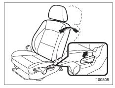
Pull the reclining lever up and adjust the seatback to the desired position. Then release the lever and make sure the seat is securely locked into place.
