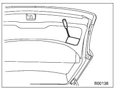
1. Use a flat-head screwdriver to remove the light cover from the top of the left-hand rear gate trim.
