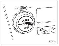
When the "AUTO" button is pressed, the indicator light "AUTO" on the display comes on. In this state, fan speed, air flow distribution, air-inlet control, and air conditioner compressor operation are automatically controlled.
