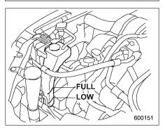
6. Pour the coolant and fill to the reservoir tank's "FULL" level mark.
