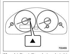
When Intelligent (I) mode is selected in vehicles equipped with a manual transmission, a shift-up indicator "A" in the tachometer will blink to signal the best time to shift gears for maximum fuel efficiency.
