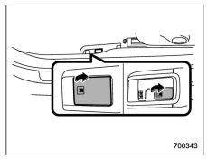
1. To open the fuel filler lid, pull the lid release lever. The lever is on the floor at the left of the driver's seat.
