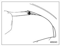
1. Remove the top of the rear gate board from the groove in the rear gate panel.
