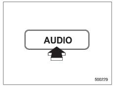
Each brief press of the "AUDIO" button changes control modes in the following sequence starting from volume control mode. (When the radio is first turned on, the control mode is in the volume control.)
