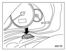
The parking light switch operates regardless of the ignition switch position.
