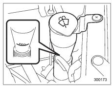
Remove the washer tank filler cap, then check the fluid level indicated by the level gauge (attached to the inside of the cap). If the level is near the "Low" mark, add fluid until it reaches the "Hi" level on the
