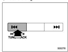
Press the "I side of the TUNE/TRACK button continuously to fast-reverse the disc/folder.
