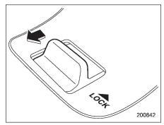
6. When you have finished entering the number, pull the lock knob to the "UN-LOCK" side within five seconds.
