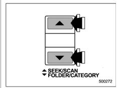
Press the "\( \bigcap \)" side of the SEEK/SCAN button to change the radio to the SCAN mode. In this mode, the radio scans through the channel until a station is found. The radio will stop at the station for five seconds while displaying the channel number, after which scanning will continue until the entire channel has been scanned from the low end to the high end. Press the "\( \bigcap \)" side of the button again to cancel the SCAN mode and to stop on any displayed channel.
