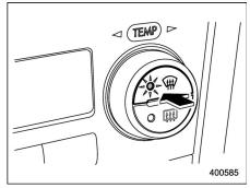
To defrost or dehumidify the windshield and front door windows, push the defroster button "\(\frac{\pmathrm{M}}{\pmathrm{M}}\)". When the "\(\frac{\pmathrm{M}}{\pmathrm{M}}\)" button is pushed, regardless whether the air conditioner is operating or not, outside air is drawn into the passenger compartment,
