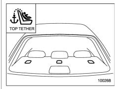
Three tether anchorages are installed on the rear shelf behind the rear seat head restraint. Open the cover flap to use each anchorage.
