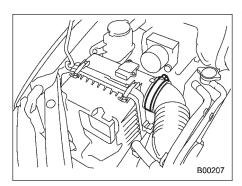
3. Use a screwdriver to remove the duct that is connected to the air cleaner case cover.
