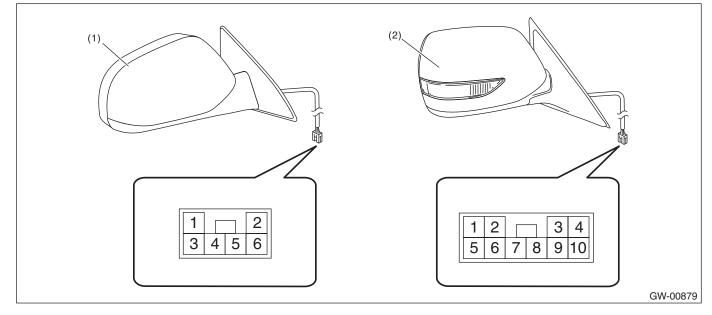
(1) Model without retractable mirror (2) Model with retractable mirror
