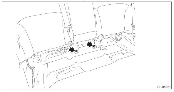
(2) Pull the release lever in the trunk room, and then tilt the backrest forward.
