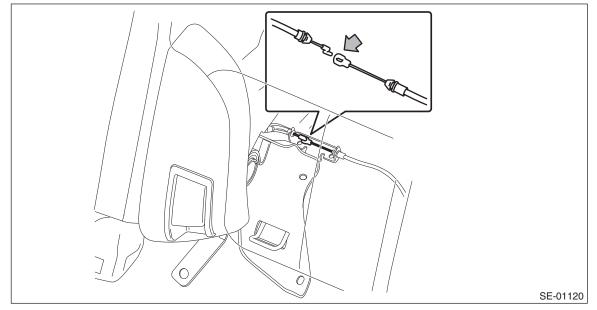
(2) Remove the screws and remove the reclining lever assembly by pulling it downward.
