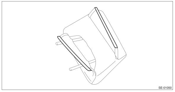
12) Remove the hog rings (A) on the rear side of the seat cushion.
