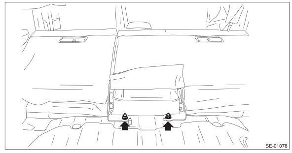
(4) Remove the backrest assembly RH from the hinge assembly RH.
