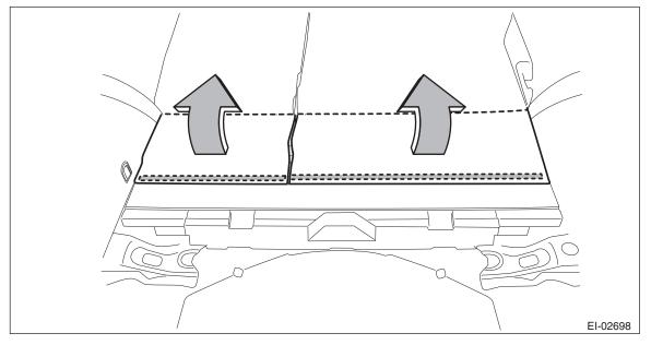
3) Remove the clips, and remove the rear floor mat-front.
