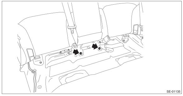
(2) Tilt the backrest forward, and then turn over the backrest backside mat.
