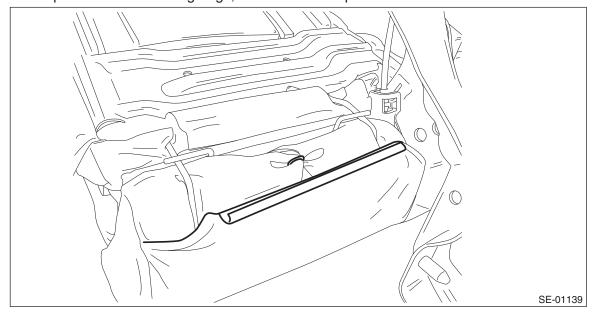
7) Remove the hog rings (A) and remove the backrest pad & frame assembly from the backrest assembly.
