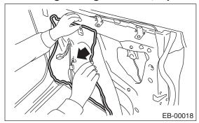
4) Release the rod from the rod clamp of outer handle.
