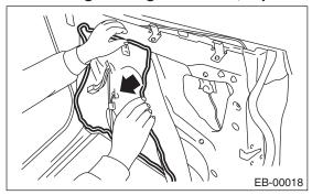
4) Release the rod from the rod clamp of outer handle.
