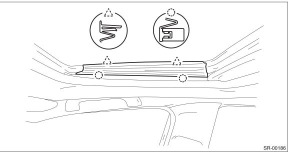
3) Remove the bolts, then remove the glass lid.
