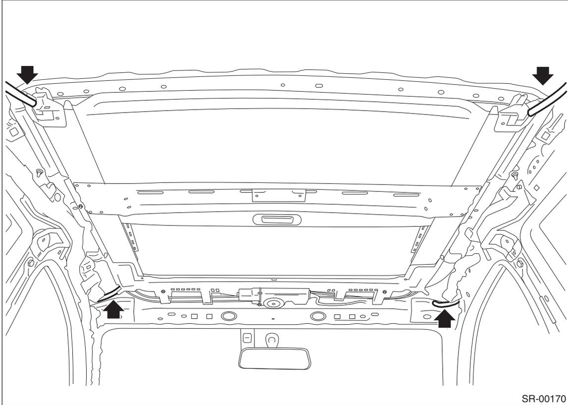
(2) Remove the bolts and then remove the sunroof bracket.
