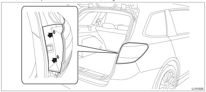
2. Release the bolts and clips, then pull out the rear combination light assembly to the vehicle rear.
