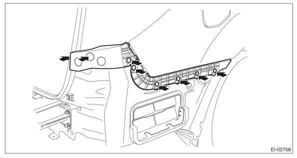
5) Remove the reflex reflector. (OUTBACK model)
