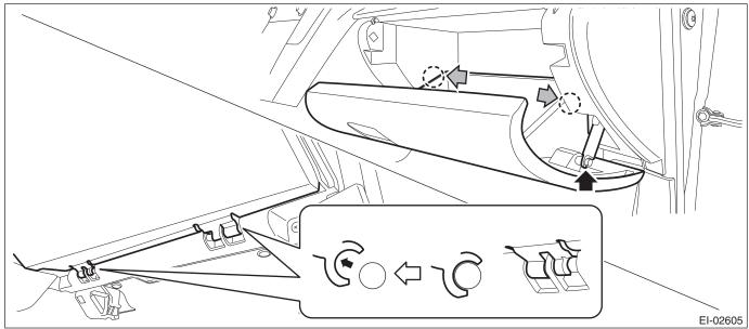
2) Release the clips, and remove the instrument panel side cover RH.
