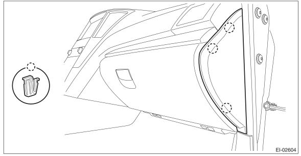
3) Remove the glove box back panel.
