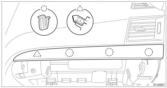
(3) Remove the screws and release the claws, then detach the glove box back panel.
