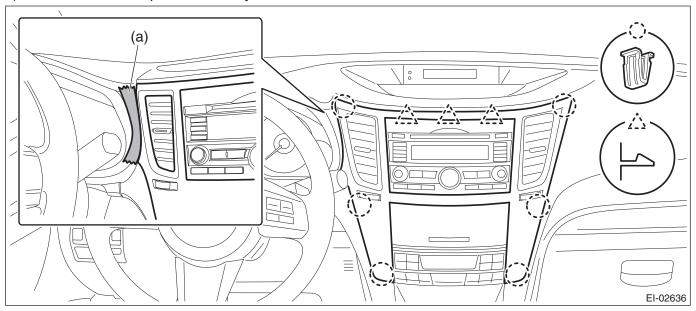
(1) Insert a finger into the air vent grille and release the left and right clips at the top of the center panel. (A), (B)
