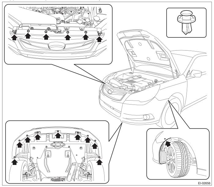
(5) Detach the flange section on the bumper face side from the bracket side front UPR.
