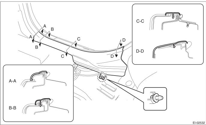
4) Release the clips and claws, and then remove the side sill cover - rear INN.
