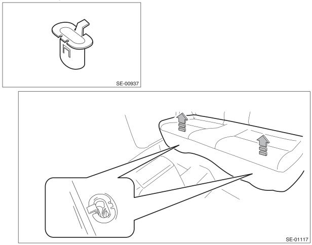
(2) Remove the hook (A) by pushing it back while lifting the front side of the seat cushion, and remove the seat cushion.
